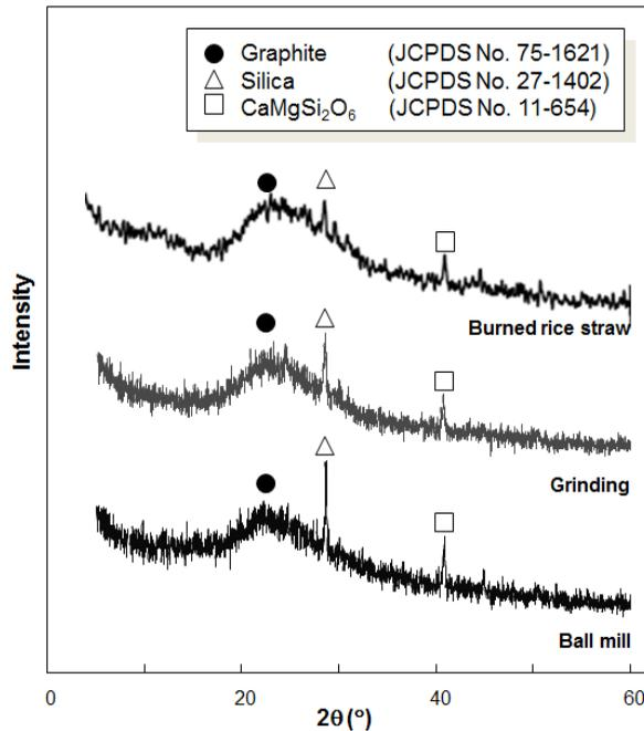
Figure 6. XRD analysis result of burnt rice straw, activated carbon by grinding, and activated carbon by ball milling
